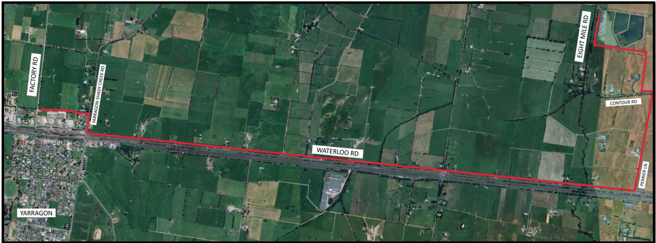
Factory Road sewerage rising main pipe alignment
